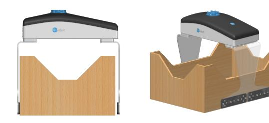
By increasing the finger height, the allowed torque might be reduced as shown in the **Moments in the finger base** section.
