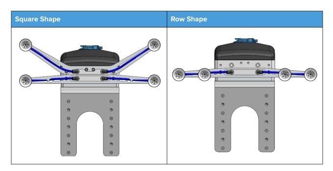
The provided tube length is adequate for the Square Shape. For using the Row Shape, please cut two of the tubes to 83 mm length.
