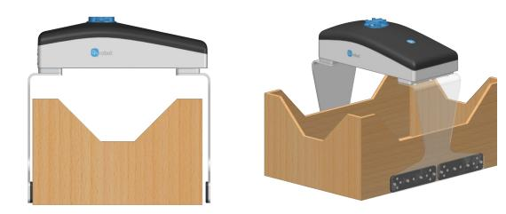
By increasing the finger height, the allowed torque might be reduced as shown in the **Moments in the finger base** section.
