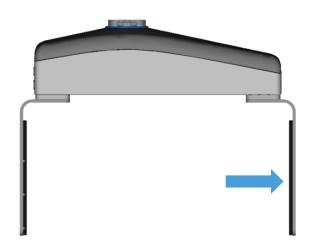
Consider the presence of the force sensor when the workpiece is aligned by using the fingers of the gripper or when the workpiece is picked sideways since the gravity can affect the force measurement.
