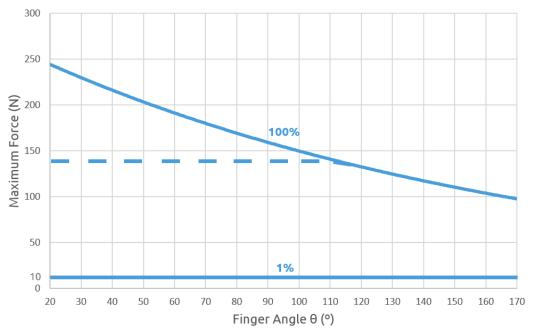
Graph plotted using measurements with 1 A current, silicone fingertips and a metal workpiece. The percetages shown on the graph stand for the target force percentage. The blue line stands for the normal Grip function and the dashed line stands for the Flexible grip function.
