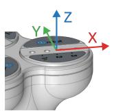
The maximum allowed torque applied to the gripper finger end around X and Y is 8 Nm.
