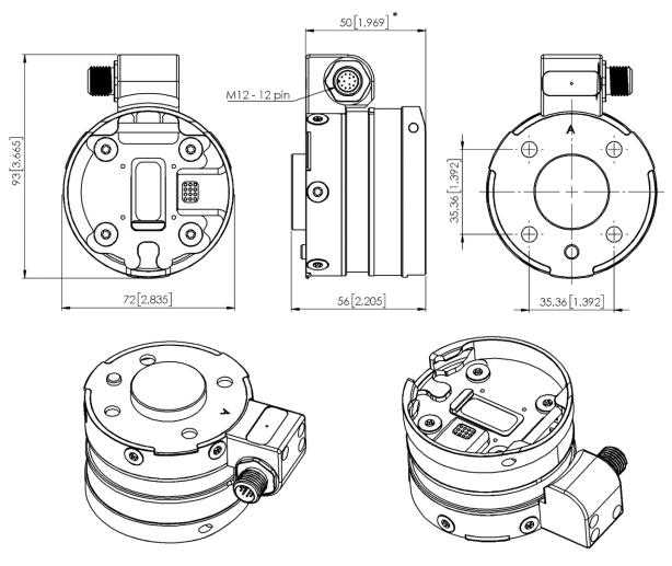
\* Distance from Robot flange interface to OnRobot tool
