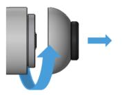
5. Ensure that the bit holder is perfectly attached by gently shaking it to make sure it is not loose.
