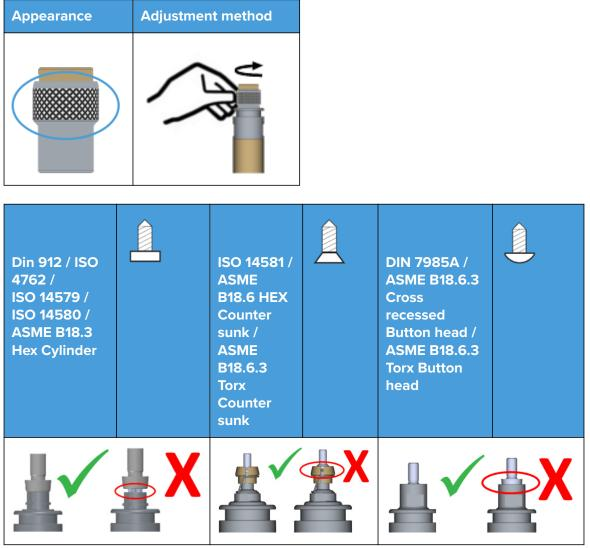
4. When this is achieved, remove the screw and push in the screw fix (only Din 912, ISO 4762, ISO 14579, ISO 14580 and ASME B18.3 HEX Cylinder screw types).
