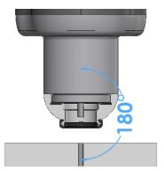
2. The distance between the Screwdriver's bottom part and the surface where the action takes place must be within the range of 0-8 mm [0-0.31 inches].
