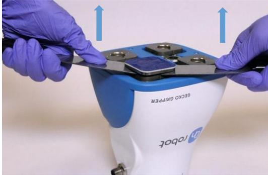
Step 3: To install new replacement pads, align the notch of the pad with the tab in the mounting hole. Push the pad into the gripper until there are no gaps between the shiny silver pad plate and backing plate.
