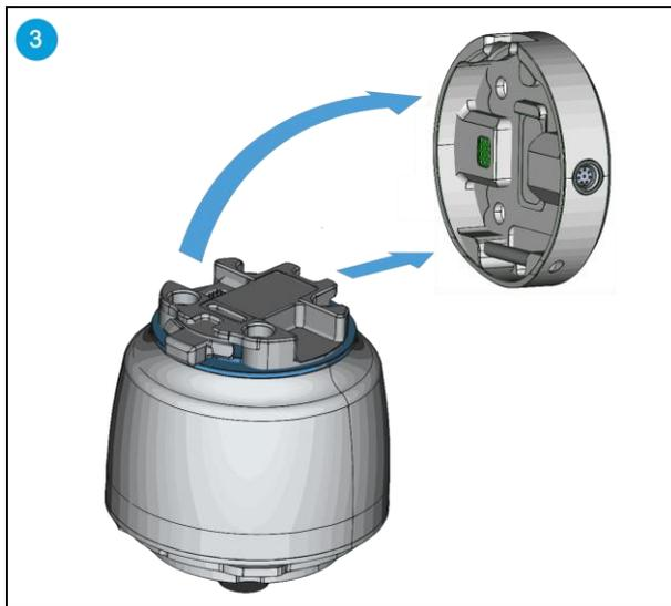
It is highly recommended to install the SG Base Part on the robot before installing the SG tool. Make sure the SG Base Part is in home position or initialized.
