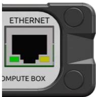
Connect the provided Compute Box (ETHERNET connector) and your computer with the supplied UTP cable.
