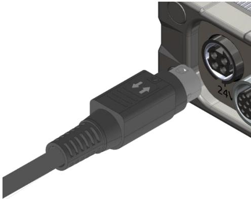
Connect the supplied power supply to the Compute Box 24V connector.
