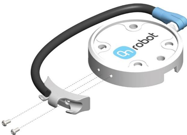
Use the M8-8pin connector on the Quick Changer or on the Dual Quick Changer.
