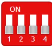
For **PNP** type set the 1. and 2. DIP switches to OFF position (down).
