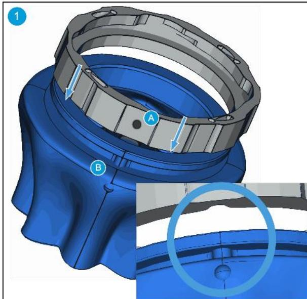
Rotate the ring so marking **(A)** facing you. Align the dot on the SG tool **(B)** with marking **(A)**. Make them fit together and mount the ring onto the SG tool.
