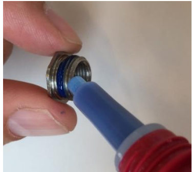
Figure 1.6: Loctite added to the Filter Fixing Fitting.
