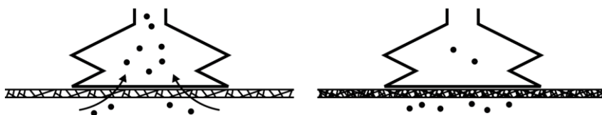
Figure 3.6: Visualization of difference in leakage through workpieces.
