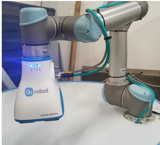
Figure 1: The Gecko Gripper mounts directly to the Universal Robot arm.
