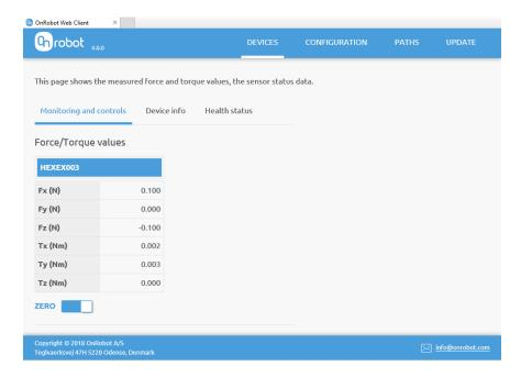
The force and torque values (Fx,Fy,Fz and Tx,Ty,Tz) are shown in Newton/Nm.
