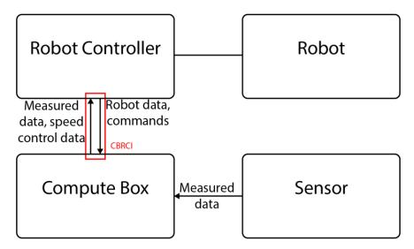
The sensor measures the force and torque data and transfers this data to the Compute Box. The Compute Box also receives data from the Robot controller about the current robot position. After receiving a command, the Compute Box performs the calculations necessary to provide instructions to the robot controller, to perform the movements that implement the commands sent by the robot controller. The instructions come in the format of speed and rotational speed values that the Robot must follow.
