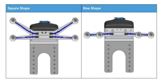
The provided tube length is adequate for the Square Shape. For using the Row Shape, please cut two of the tubes to 83 mm length.
