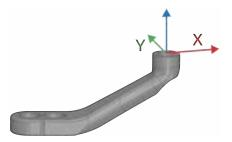
The pictures above show the coordinate system from where the maximum allowed torques are calculated.
