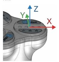
The maximum allowed torque applied to the gripper finger end around X and Y is 2.5 Nm.
