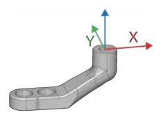
The pictures above show the coordinate system from where the maximum allowed torques are calculated.
