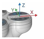
The maximum allowed torque applied to the gripper finger end around X and Y is 8 Nm.
