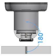
2. The distance between the Screwdriver's bottom part and the surface where the action takes place must be within the range of 0-8 mm [0-0.31 inches].
