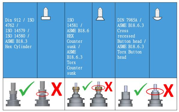
4. When this is achieved, remove the screw and push in the screw fix (only Din 912, ISO 4762, ISO 14579, ISO 14580 and ASME B18.3 HEX Cylinder screw types).
