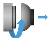
4. Place the hex shape of the bit holder inside of the end of the Screwdriver's shank. The system will be attached to the Screwdriver by a magnetic force.
