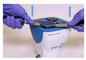
Step 3: To install new replacement pads, align the notch of the pad with the tab in the mounting hole. Push the pad into the gripper until there are no gaps between the shiny silver pad plate and backing plate.
