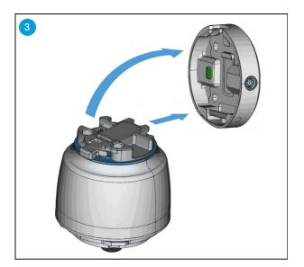
It is highly recommended to install the SG Base Part on the robot before installing the SG tool. Make sure the SG Base Part is in home position or initialized.
