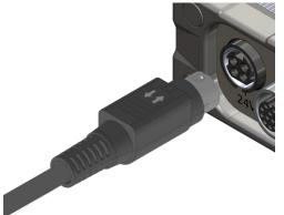
Connect the supplied power supply to the Compute Box 24V connector.
